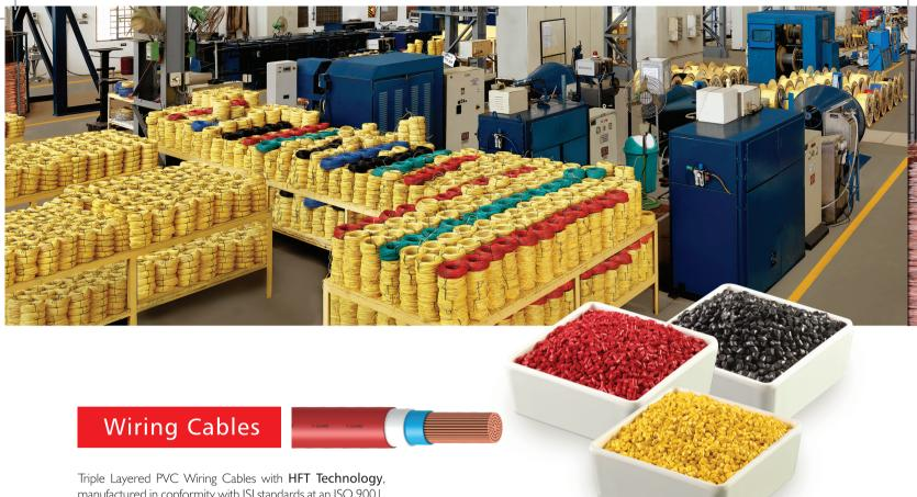
manufactured in conformity with ISI standards at an ISO 9001, ISO 14001 & OHSAS 18001 certified manufacturing plant, V-Guard wires ensure triple protection for every home. The high quality online annealing prevents breaking of the copper strands when bent or twisted, making V-Guard wires protect homes like nothing else.
